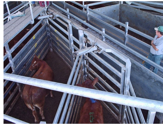
Pneumatically-swung gates used in stacking pens.
