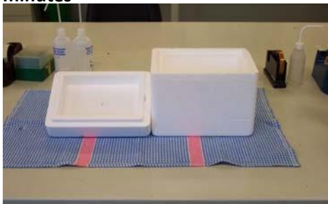
Picture 3. Thick walled eskie used to maintain samples at 95oC for 30 minutes
