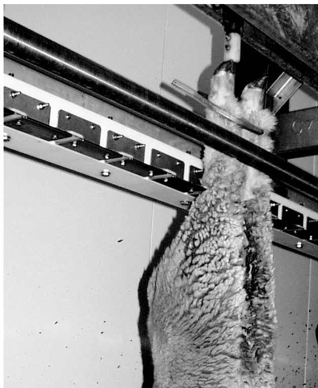
Fig. 2. Photograph showing a predressing electrical stimulation unit with the current administered through the skin on back legs.
