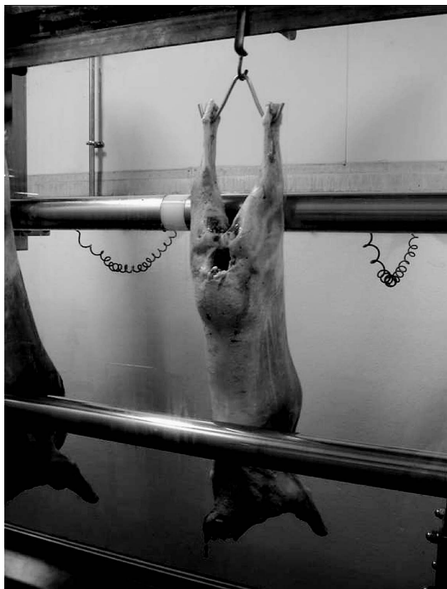
Fig. 3. Photograph showing a postdressing electrical stimulation unit – the separate electrodes can be seen separated by the white insulator and only one carcass is in contact with any one electrode at any one time.
