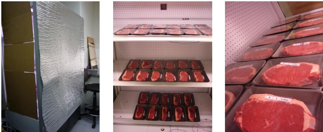
Figure 9: Far left: retail display cabinet covered to minimise interference from external light. Centre: cabinet containing steaks across all 3 shelves and top shelf (far right).
