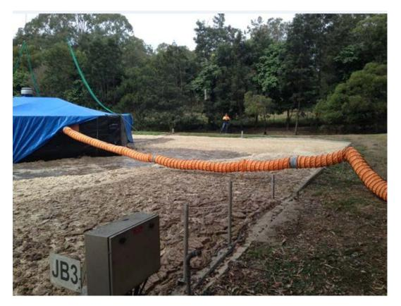
Photo 5: Pilot test rig setup over the aerobic ponds ready for odour collection.
