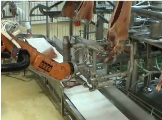
Step 1 – Primal system (Tower 1) removes forequarter from carcass
