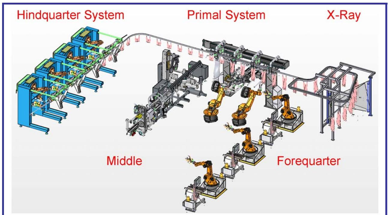
This project aimed to, and successfully developed and demonstrated, a forequarter processing module via development of a lab prototype.
