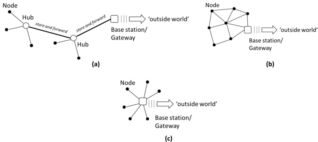
Figure 2-3. A basic network diagram as relates to (a) 'store and forward', (b) 'mesh', and (c) star farm sensor networks (Extracted from Lamb, 2017).
