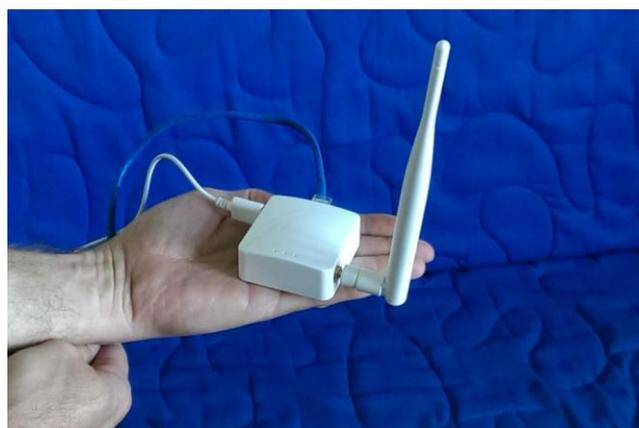
**Figure 2-8. An example of a low-cost Wi-Fi node capable of forwarding internet access as deployed in a community WYSPS mesh network (Extracted from Lamb, 2017).**
