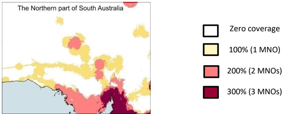
Figure 3-7. Map of coverage overlap in a segment of South Australia (Source: Lamb, 2015).
