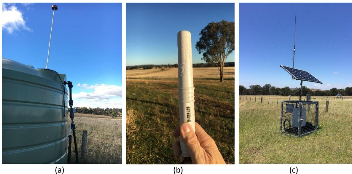
*Figure 2-9. (a) A water tank sensor and transmitter, (b) close-up of low power transmitter and (c) Taggle LR/LP base station receiver (vertical aerial) and mobile network gateway (small white ‘bulb’ antenna located on protection cage) (Extracted from Lamb, 2017).*
