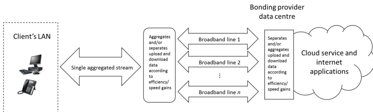
Figure 3-20. Schematic of broadband bonding (Extracted from Lamb, 2017).
