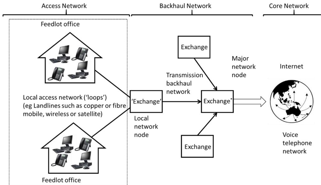
Figure 3-1. Schematic diagram of a basic network structure (Extracted from Lamb, 2017).
