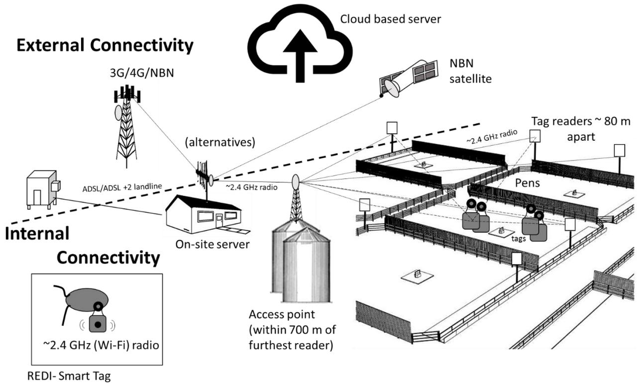
Figure 6-4. A schematic showing connectivity between REDI smart tags and internal and external system
