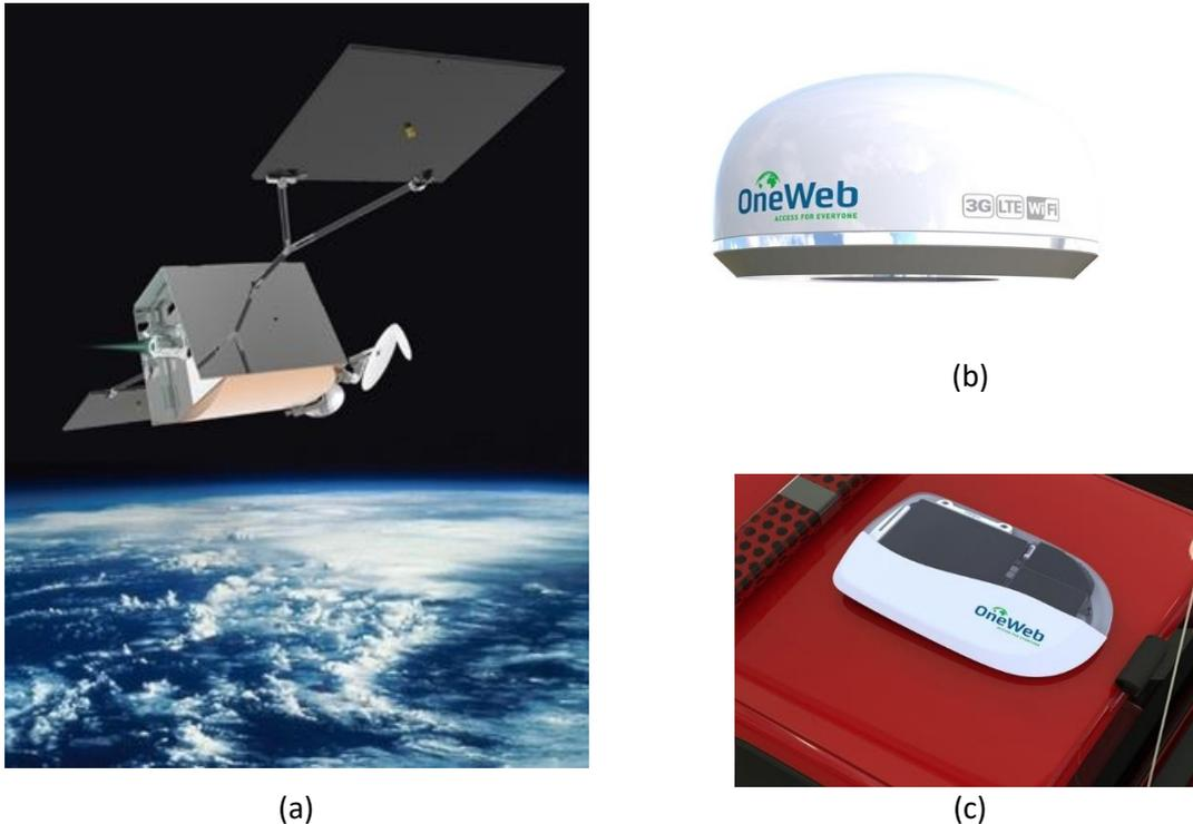
Figure 5-2. (a) Graphic of one of the proposed 648 LEO telecommunications satellites to be launched by U.S company OneWeb, (b) a user terminal for a building and (c) for a vehicle. Once linked to the LEO satellites, these act as a small cell, generating a 3G or LTE (and Wi-Fi) zone around it for an existing mobile network operator (Source: <http://oneweb.world/#technology>) (Extracted from Lamb, 2017).
