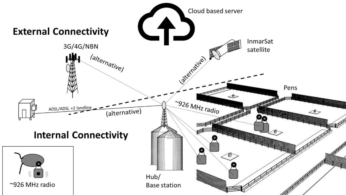
Figure 6-2. A schematic showing connectivity between smart tags and internal and external systems (Source: Stewart McConarchy).
