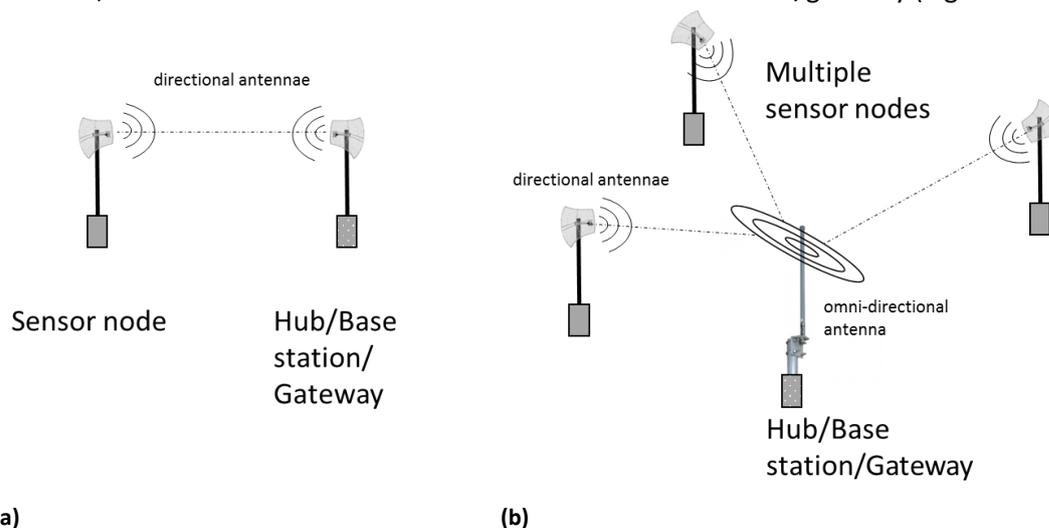
Figure 2-5. A basic wireless sensor network (WSN) indicating use of different antenna types used in (a) point-to-point and (b) point-to-multipoint links (Extracted from Lamb, 2017).
