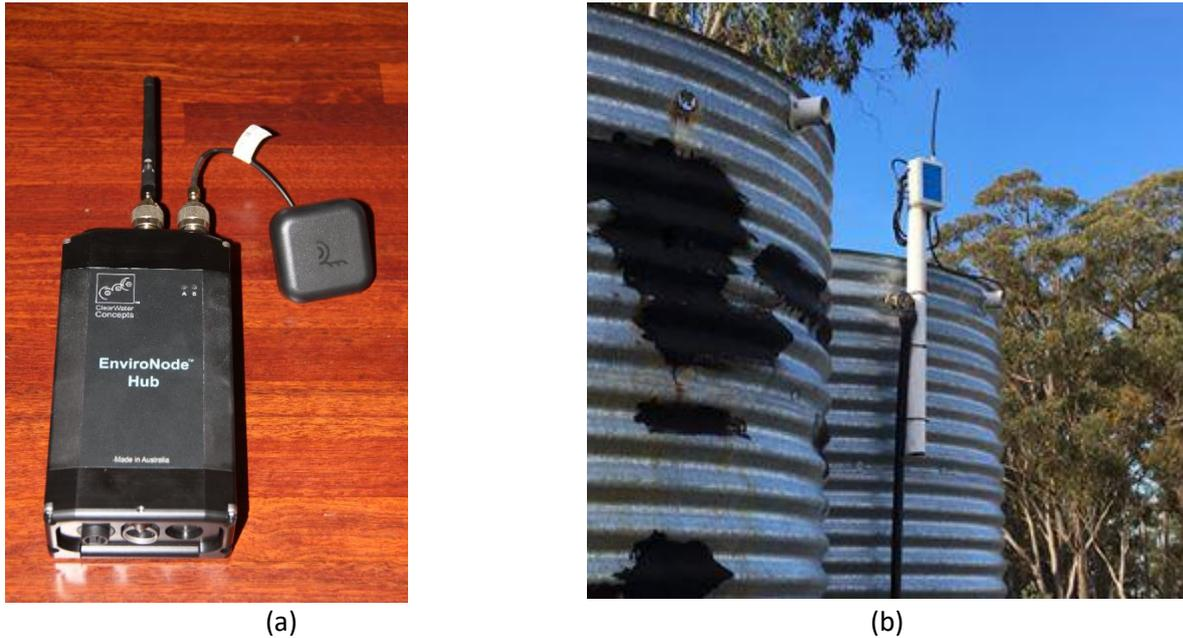
Figure 3-16. (a) An example of an Iridium IoT hub and (b) a Myriota-developed LEO satellite transmitter connected to a tank water level sensor. (Source: Ric Otton, Dosec Design and Tom Rayner, Myriota; extracted from Lamb, 2017).
