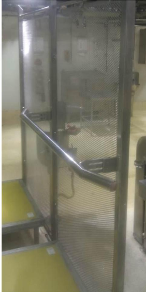
**Fig.6 Perforated Stainless steel guarding**
