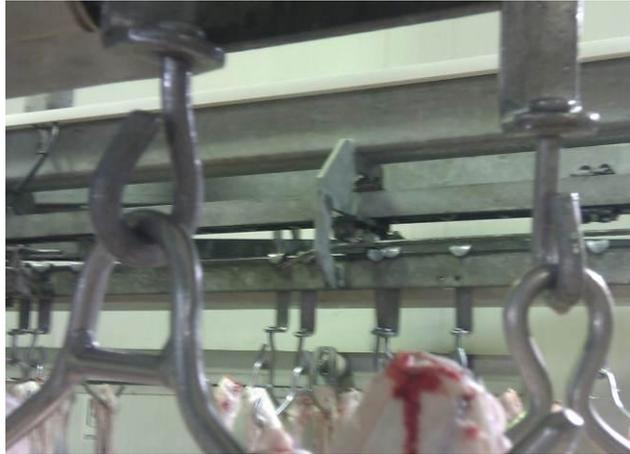
**Fig.23 Different length of flat bar on gambrels used at JBS Brooklyn**
