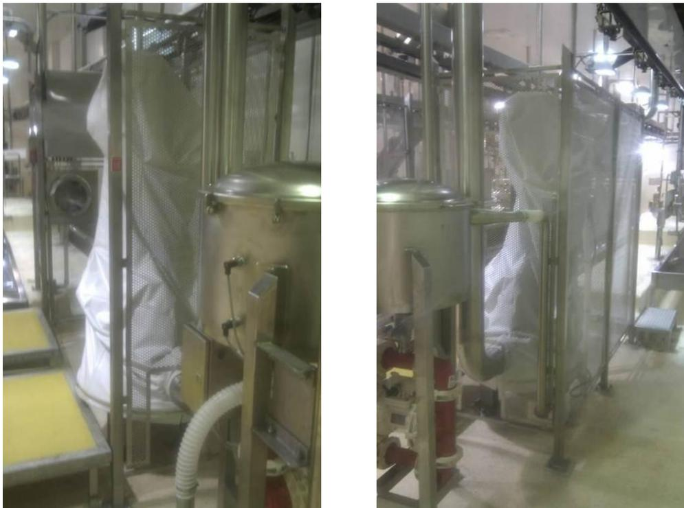
**Fig 5 External views of cell showing guarding and cyclone tank**
