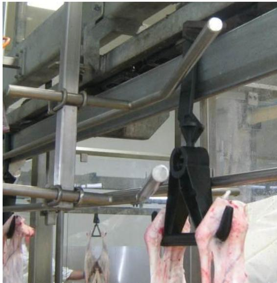
**Fig.17 Gambrel and Carcass stabilization as used at Peel Valley**
