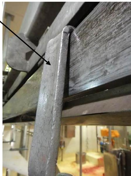
**Fig. 20 Initial gambrel Stabilization used at JBS Brooklyn**
