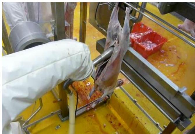
**Fig.18 Carcass support bar at Peel Valley to prevent excessive movement of the carcass during fat removal**
