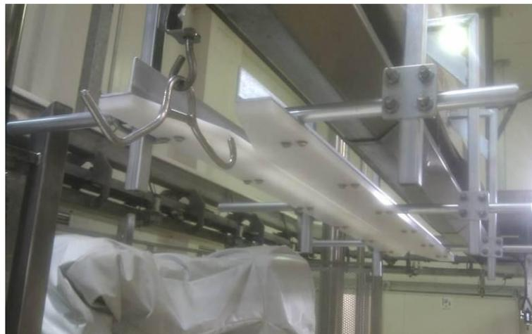
**Fig.22 Second stabilization mechanism trialed**
