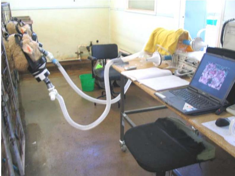
**Image 3.** Indirect calorimetry equipment and measuring sheep for respiration
