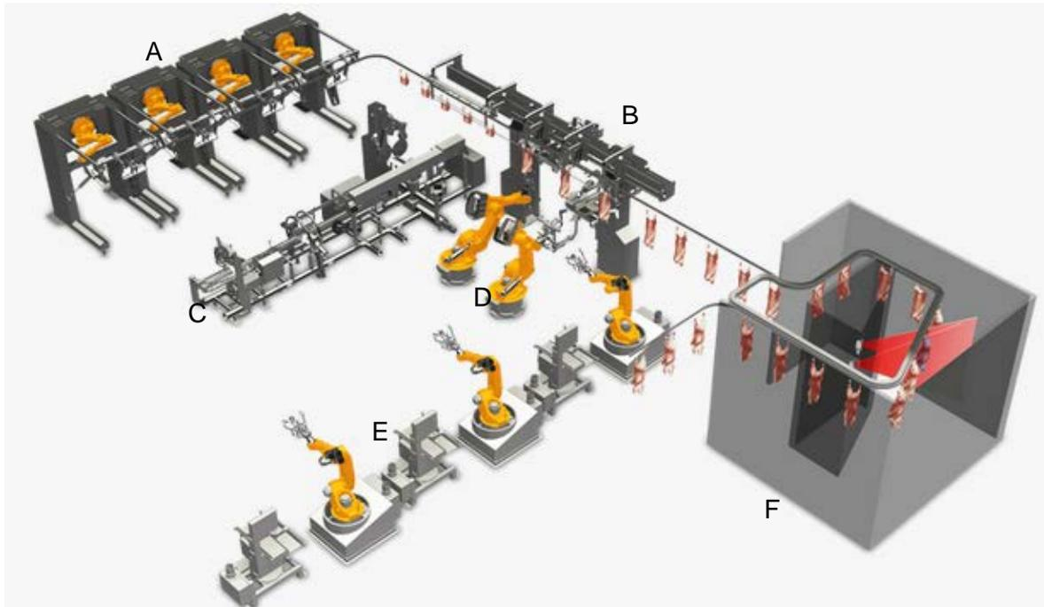
**Figure 1: Scott Vision (now realised) of a fully automated bone-in lamb processing facility (Legend: A: hindquarter, B: Primal, C: middle, D: integration robots, E: forequarter, and F: x-ray system)**
