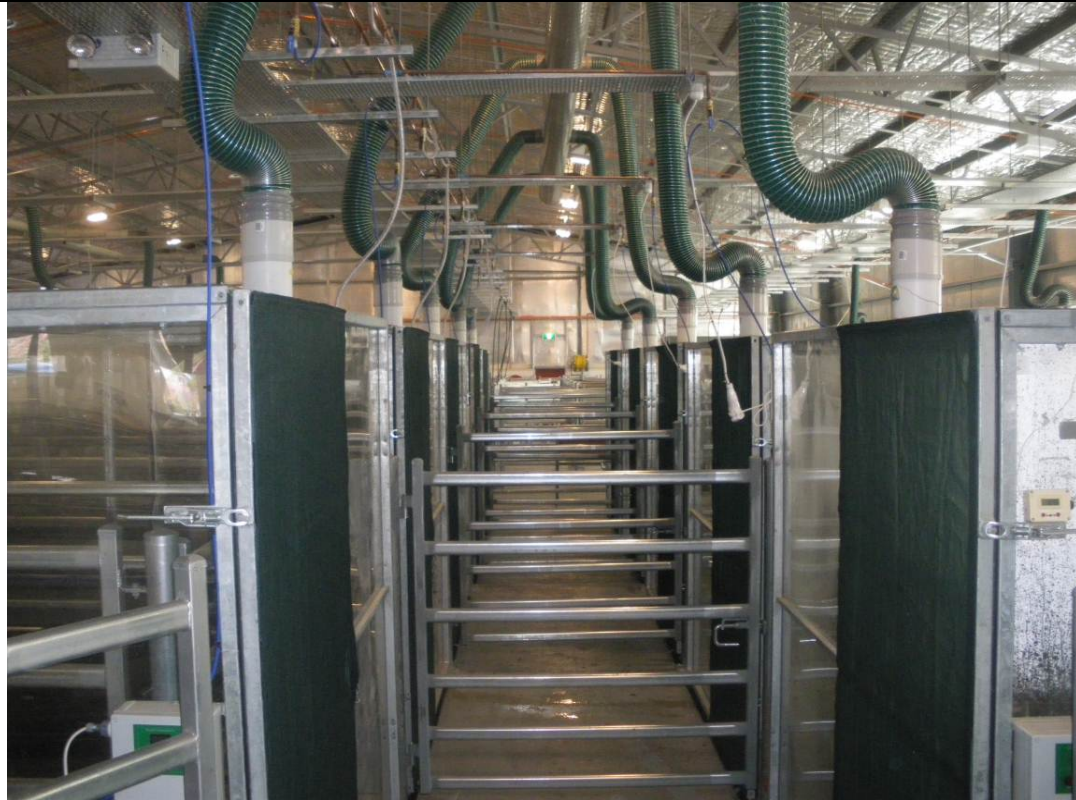
Figure 4. Open circuit cattle respiration chambers used in this study. Cattle were fed a matching intake to what they had consumed over the previous 2d in the yards, however there were refusals in most cases which will complicate the chamber:GEM comparisons.
