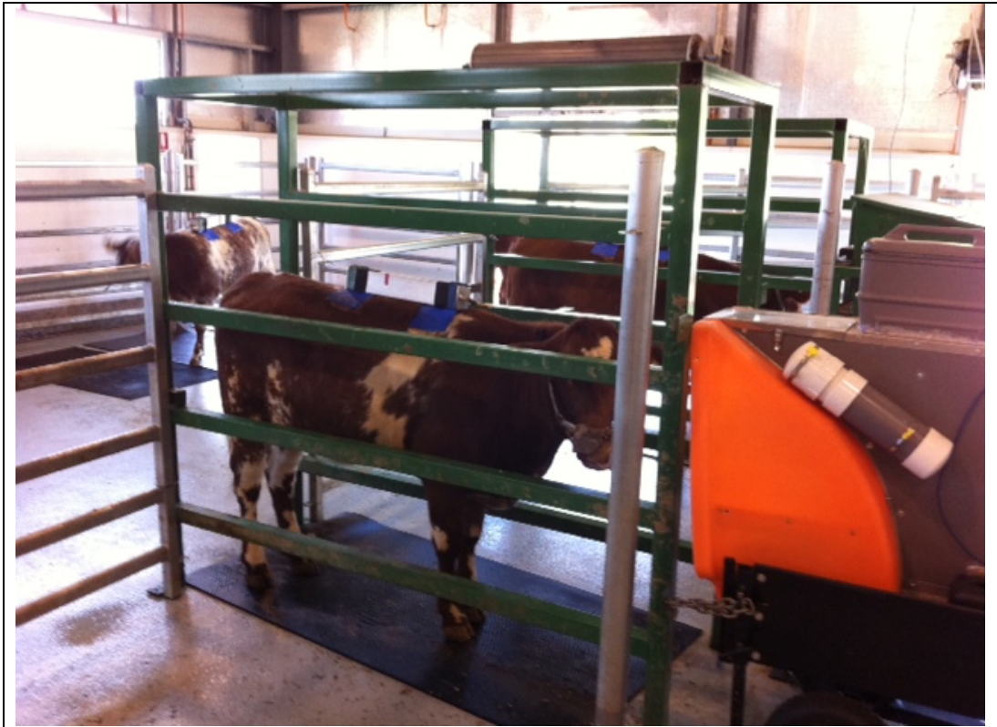
Figure 3. Heifer with SF 6 collection canister mounted on her back while accessing the GEM water dispenser
